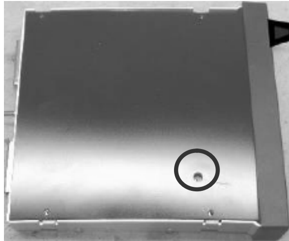
Figure 2-5 – Unswitched 3 Audio Level (bottom cover removed)
