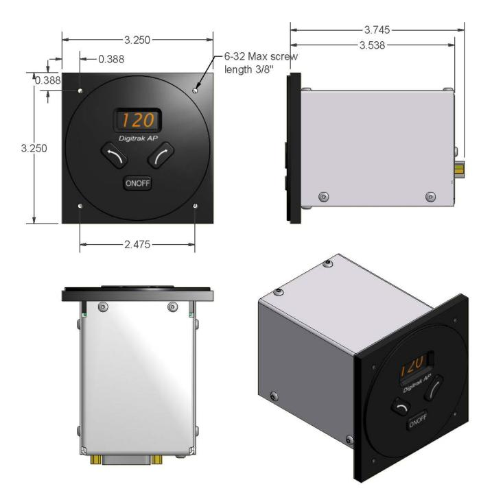
MOUNTS IN STANDARD 3 1/8" INSTRUMENT HOLE
