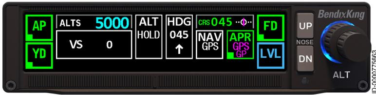
Figure 31 GPS Approach With Glide Path, Steps 6-7
