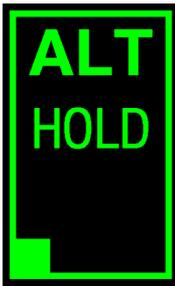
Pressing the **ALT HOLD** button again toggles the Altitude Hold mode, reverting to Pitch mode. The Altitude Hold mode can also be turned on when Altitude Hold mode is Armed, and the target altitude is captured by the autopilot.
