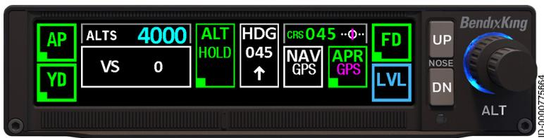
Figure 32 NAV GPS Manual Step-Down, Steps 1-3
