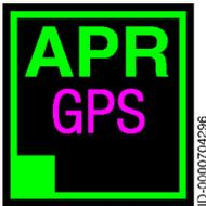
When the pilot selects APR mode by pressing the **APR** button, the autopilot engages either APR Arm or APR Capture mode, depending on course proximity and closure rate. Roll or Heading mode can be active with APR armed, but these lateral modes disengage as soon as the APR capture sequence begins.
