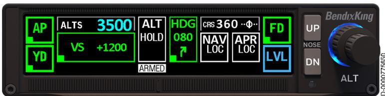
Figure 18 Takeoff and Climb to Assigned Altitude, Step 3-5
