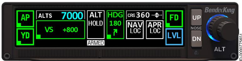
Figure 19 Turn and Climb to Assigned Altitude, Steps 1-4
