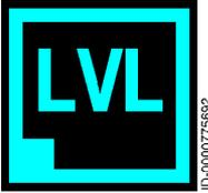
With the straight and level mode functionality, the autopilot provides a way to return the aircraft to straight and level trim condition. Straight and level mode can be engaged by pressing the **LVL** button. Once engaged, both the autopilot and flight director are activated.
