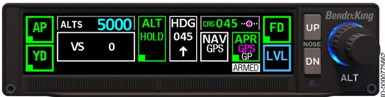
Figure 30 GPS Approach With Glide Path, Steps 1-5
