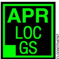
The text inside the button depicts the APR source and the type of source (VOR, LOC, LOC BC, GPS) and a vertical guidance source (+GP, +GS), if applicable. Active radio-based navigation sources display green. Active GPS-based navigation sources display magenta.
