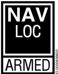
When NAV mode is inactive but available, **NAV** is annunciated on the touchscreen by white text and a white border. The arming of NAV mode is displayed by an **ARMED** label under the NAV button on the autopilot screen. When the NAV course is captured, the **ARMED** label is removed, and the **NAV** button transitions to **NAV** and flashes in green for 5 seconds, remaining green until another mode is commanded.
