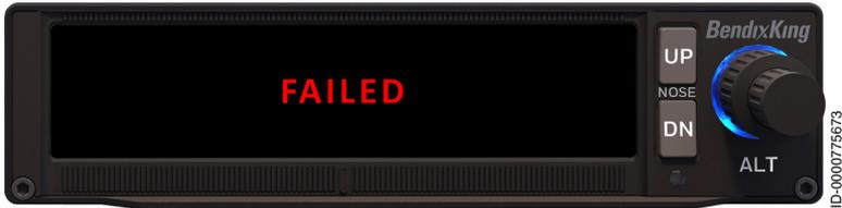
Figure 40 System Failure 10-Second Flash
