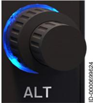
The Altitude Selector knob allows the pilot to select an altitude, displayed to the right of the ALTS display, for the autopilot to capture and engage in Altitude Hold mode.
