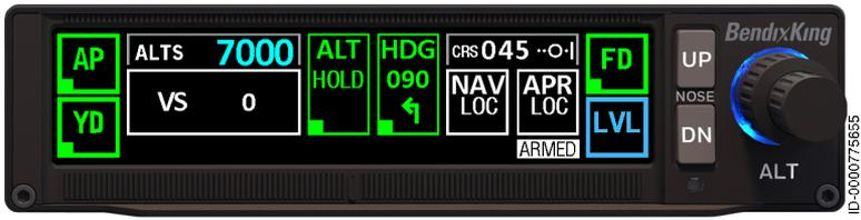
Figure 23 Localizer Inbound for Procedure Turn to ILS Approach, Steps 4-7
