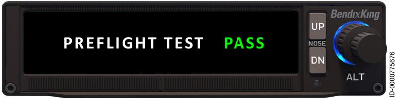
Figure 6 KFC 230 Successful Preflight Test
