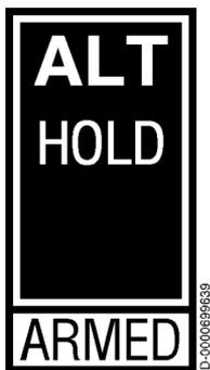
When a new altitude is selected, and the aircraft is in a vertical path mode (Vertical Speed (VS) or Pitch) toward the selected altitude, Altitude Hold (ALT HOLD) mode arms to capture the new altitude.
