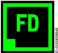
While hand flying, the flight director provides guidance to fly the trajectories computed by the autopilot to meet either pilot-specified (Vertical Speed, Heading, etc.) or default mode (Pitch, Roll) targets. With the autopilot engaged, the flight director allows the pilot to monitor the autopilot performance.
