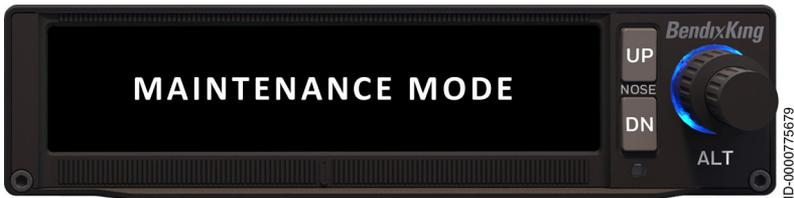
Figure 10 KFC 230 Maintenance Mode
