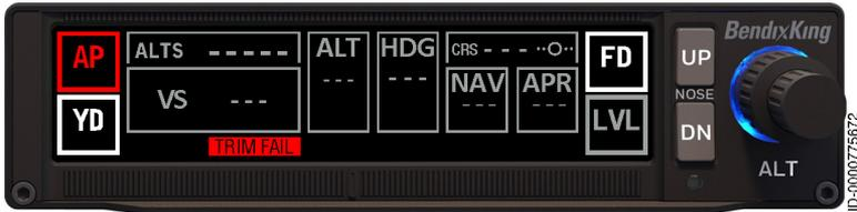
Figure 43: Trim Failure
