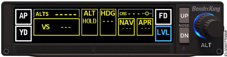
Figure 36 Failed Annunciation
