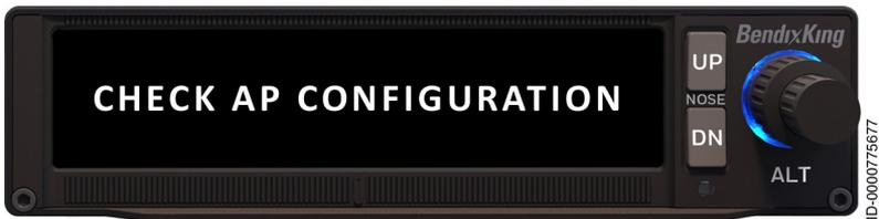
Figure 8 KFC 230 Check AP Configuration
