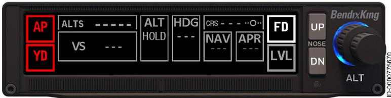
Figure 38 Servo Failure
