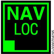
When the pilot selects NAV mode by pressing the **NAV** button, the autopilot engages either NAV Armed or NAV Capture mode, depending on course proximity and closure rate. Any of the lateral modes can be active with NAV mode armed, but these lateral modes disengage as soon as the NAV capture sequence begins.
