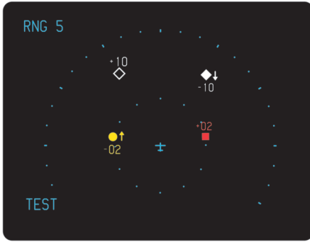
CAS 67A Radar Test Pattern; 5NM range
