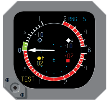
CAS 67A TA/VS I Test Pattern; 5NM range
